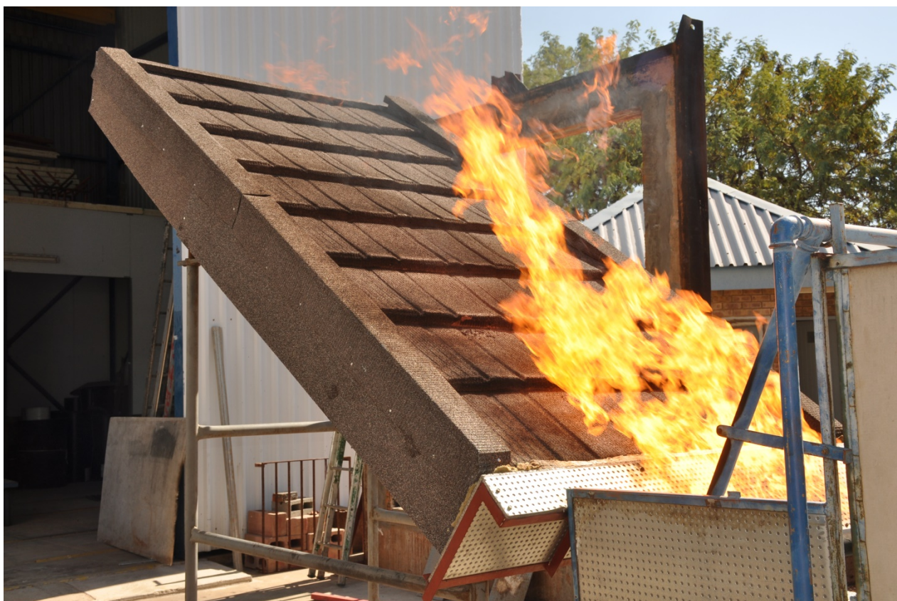
Figure 4.1.4: Harvey Thatch Tile Roofing System during final cycle of Intermittent Flame Exposure Test
