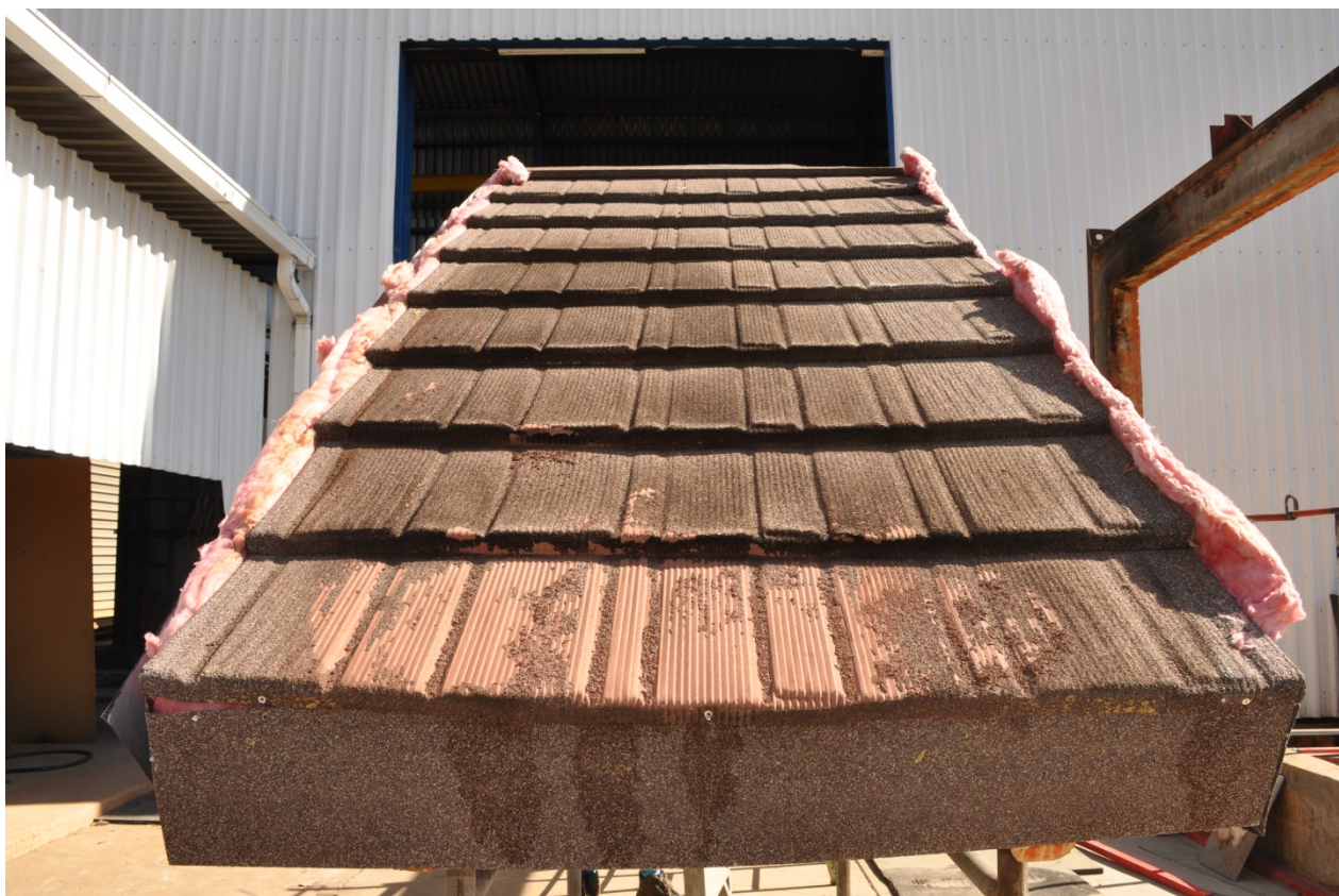
Figure 4.1.7: System with eave tiles removed – Slight discolouration to Pink Aerolite
