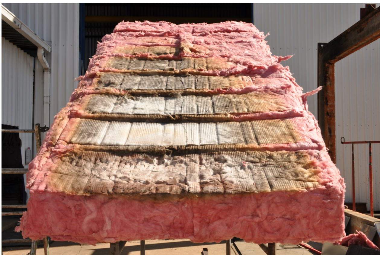
Figure 4.1.8: Condition of the Pink Aerolite covering Pine Brander below Harvey Thatch Tiles
