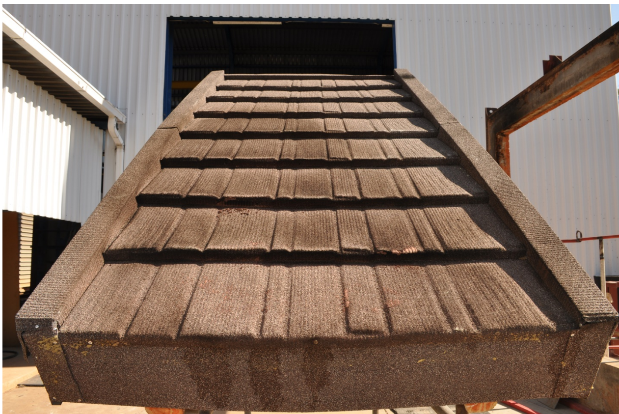
Figure 4.1.5: Exposed surface of Harvey Thatch Tile Roofing System after conclusion of test
