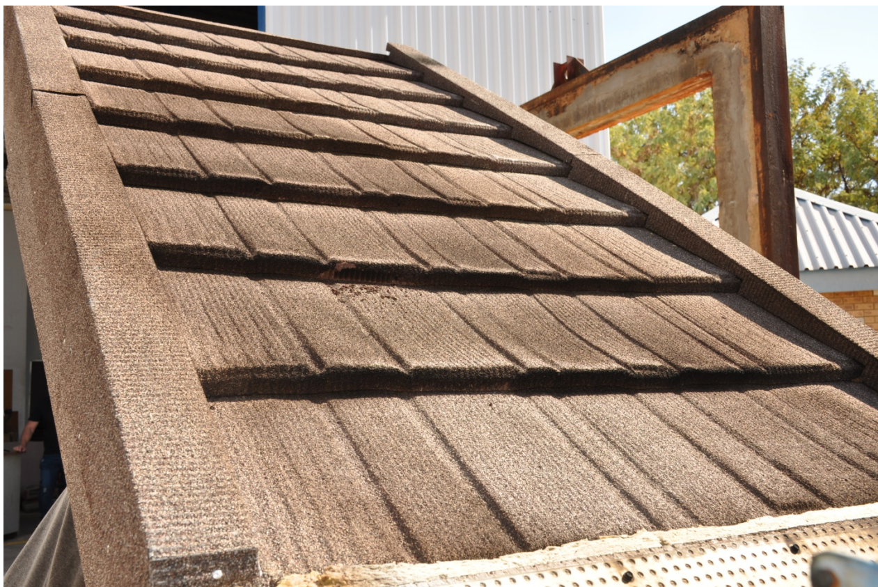
Figure 4.1.3: Deformation of Harvey Thatch Tiles (Buckling downwards)
