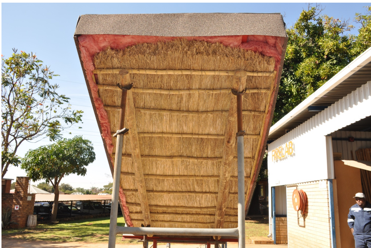
Figure 4.1.6: Unexposed interior surface of thatch roof after conclusion of test
