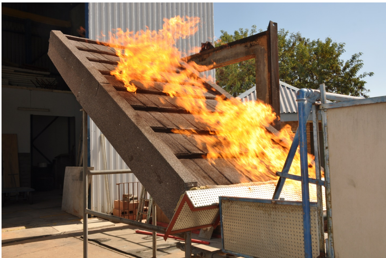
Figure 4.1.1: Start of Intermittent Flame Exposure Test
