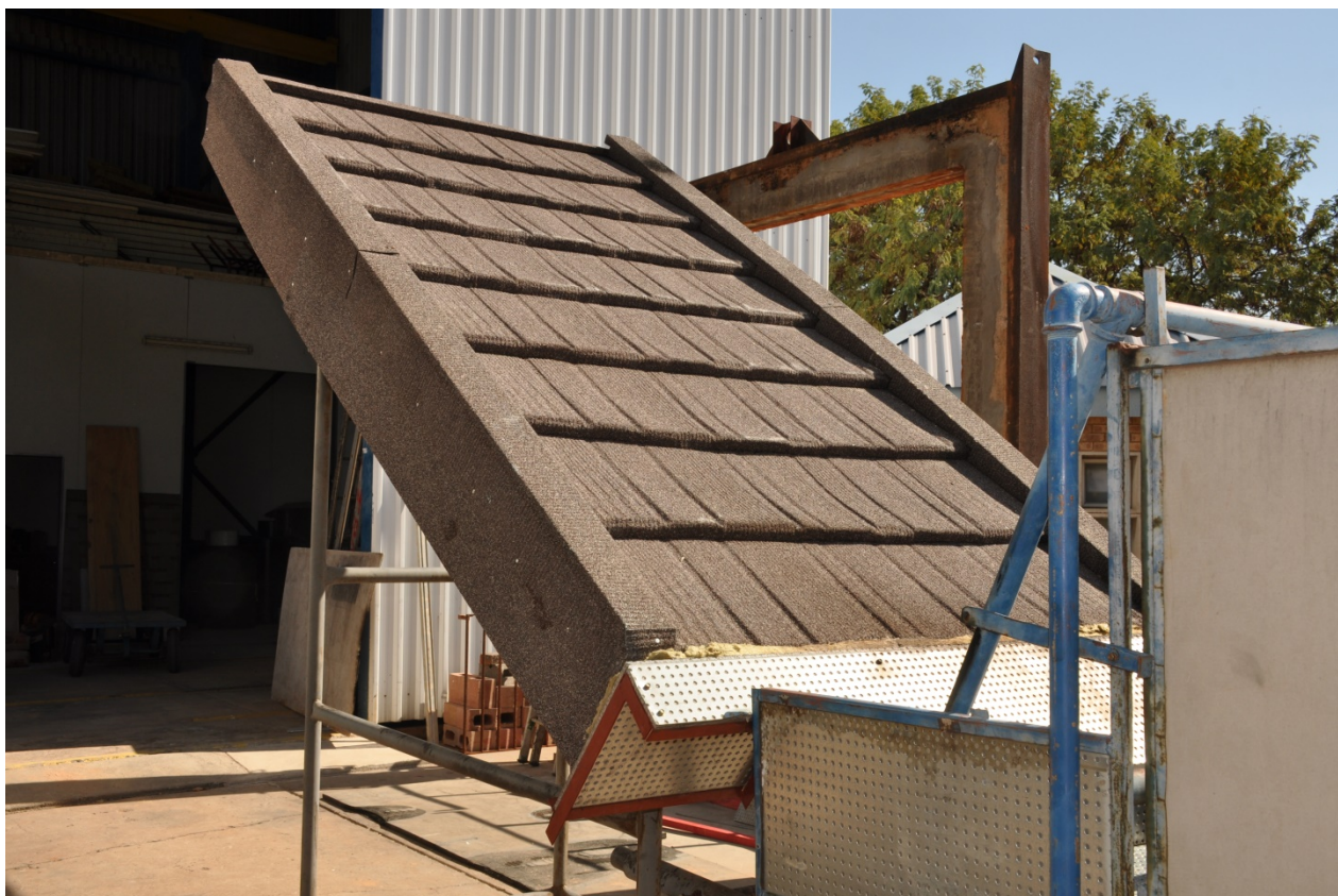
Figure 2.1: Harvey Thatch Tile Roofing System on a treated thatch roof prior to test
